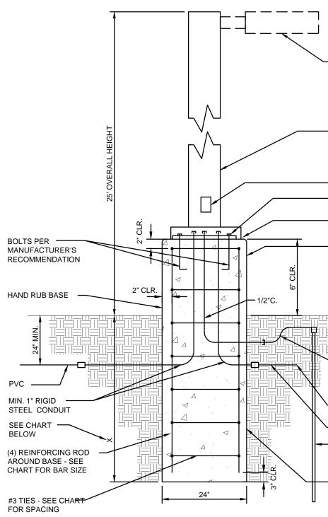
NOTES: A DRILLED 2'-0" DIA. HOLE SHALL BE USED AS THE FORM FOR THE CONCRETE BASE IN UNDISTURBED EARTH, EXCLUDING FILL MATERIAL. BACKFILL AROUND CONCRETE BASE WITH COMPACTED GRANULAR BACKFILL A MIN. OF 2'-0" IN ALL DIRECTIONS IN EXCAVATED AREAS OR IN EXISTING SOIL CONTAINING FILL OF OBJECTIONABLE MATERIAL DESIGN BASED ON IBC-2009: 100 MPH WIND SPEED, EXPOXURE C, 150 PSF/FT LATERAL SOIL
