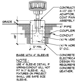
ADAPTOR, POWDER COAT PAINT AFTER ASSEMBLY. -COUPLER
